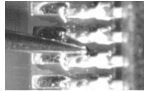
25 MilProbe used to test solder joint of 30 mil pitch QFP.
